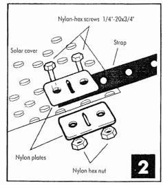
When you install the attachment kits, it must be at equal distance amongst them. The length of the attachment must be adjusted in regards with the shape of the pool.
