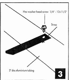
You must drill holes in aluminium tubing to fix straps which are already attached to sollar cover.
